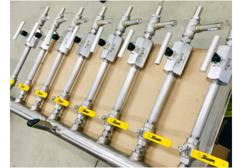
Large Return Manifold Assembly with Electronic Pressure Sensors, Pipe for Non-Contact Flowmeters, Needle Valves and Hammer Arrestors for Server Cooling Application
