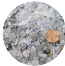
PET Flake w/Aluminum (4mm-10mm) 96% Aluminum Contamination Removed
