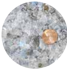
PET Flake w/Aluminum (<4mm) 93% Aluminum Contamination Removed
