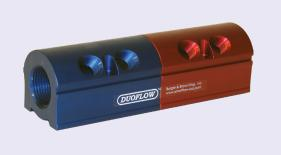
**SWAP Valves** reduce time required for cooling line evacuation between mold changes to seconds instead of minutes while keeping shop floors clean. SWAP valves use shop air to evacuate fluid from cooling lines with a single handle motion. The mold can then be changed. Resume main cooling fluid supply with the reverse handle motion.
