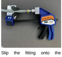
Slip the fitting onto the mandrel and begin moving the the movable section by squeezing the blue and black handles. Align the fitting into the end of the hose, continue slowly squeezing as the fitting is pressed into the hose up to the plastic washer.
