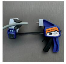
Slip the hose between the two spring loaded jaws with about 2 times the fitting barb length protruding beyond the jaws.
