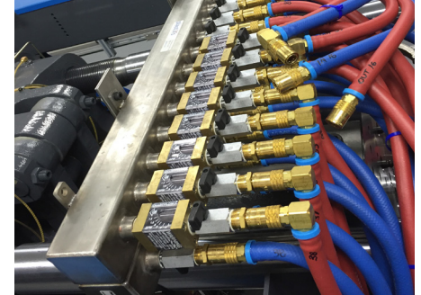
Compact Stainless Steel Manifold Assembly with Flowmeters, Mini Ball Valves, and Brass Fittings for Injection Molding
