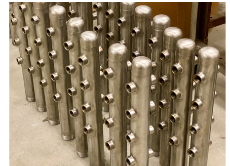
Tee Manifolds Awaiting Assembly for Brass Ball Valves. Application for Welding Gases for Car Manufacturer's Welding Robots (over 400 produced)
