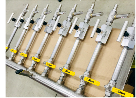
Large Return Manifold Assembly with Electronic Pressure Sensors, Pipe for Non-Contact Flowmeters, Needle Valves and Hammer Arrestors for Server Cooling Application
