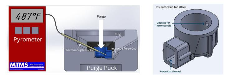
NOTE: A minimum of 1 ounce purge is required for accurate melt temperature measurement.
