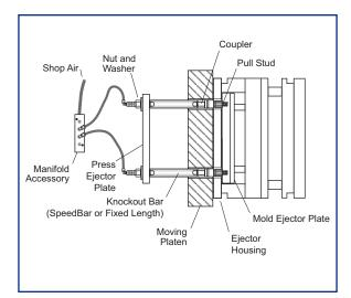
This setup is designed for captive molders, or shops with tools using a standard ejector stroke.
