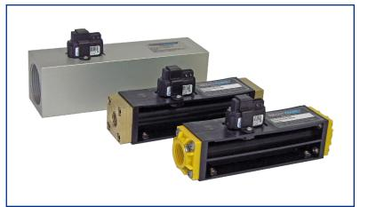
Connection to the process is made using standard pipe threads in NPT or BSP from 3/8" through 1-1/2". Flow body materials are corrosion-resistant brass, nylon, anodized aluminum and stainless steel. Options are based on thread size, see page 2 for details.
