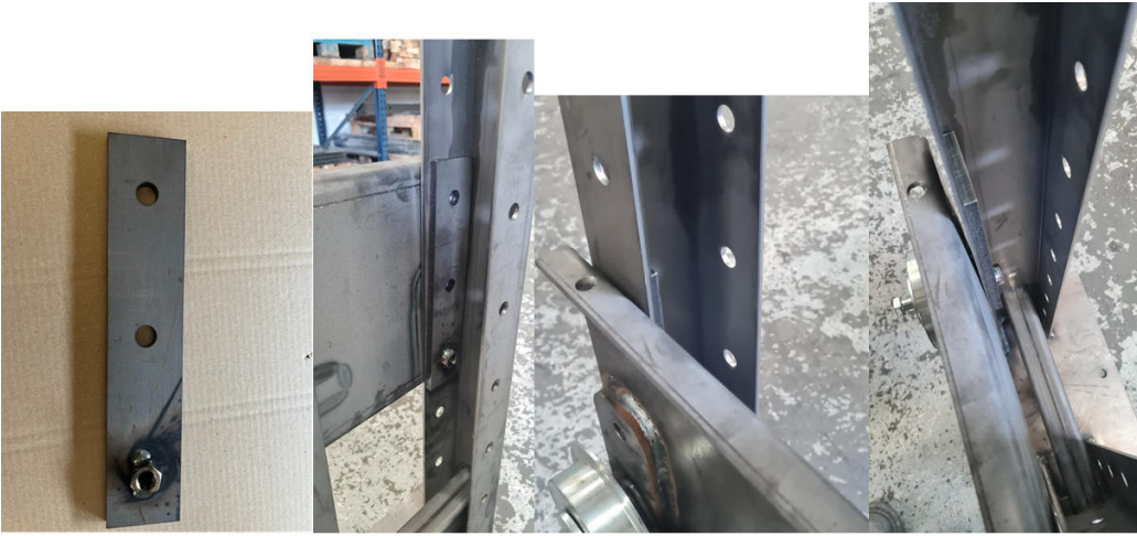
Reinforcement Plate for 100% pull-out tracks. One plate inside of the channel, behind the track and post wheel
