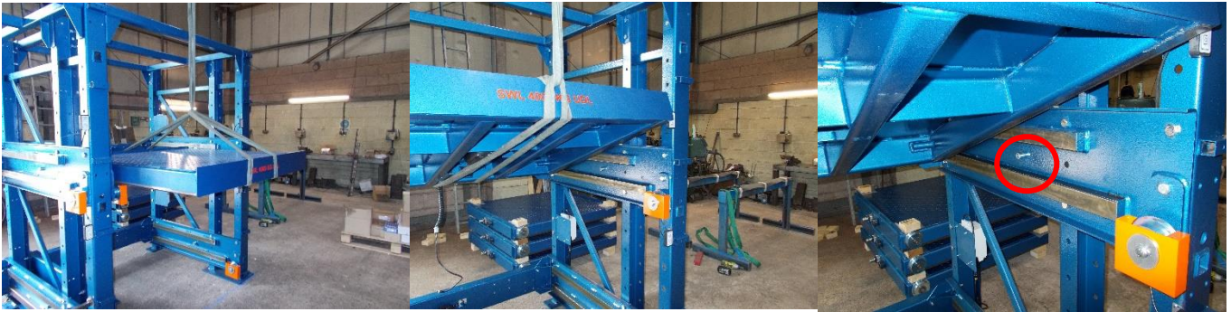
Stop bolt with laser cut washer. Critical – must be in position before lowering shelf
